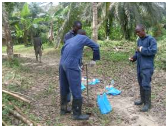
Soil Sampling using hand Auger
