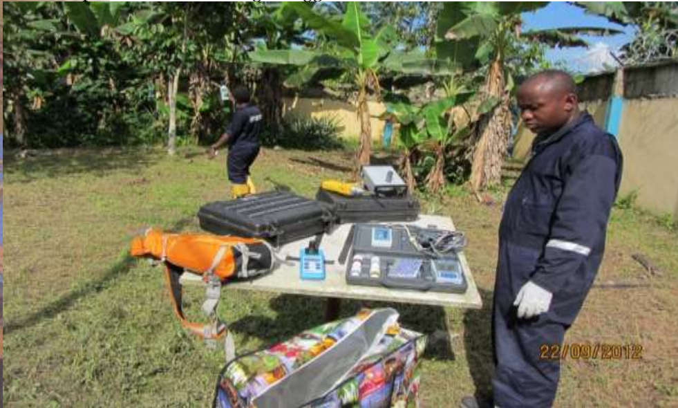
In-situ measurement of ground water samples
